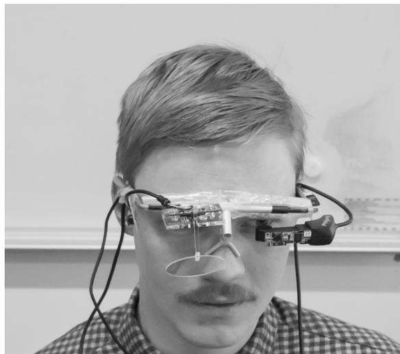
Fig. 1. A subject wearing the eyewear setup including the gaze tracker (tracking the right eye) and a HMD on the left eye. A head tracker sensor is mounted on the right side of the Glasses frame.
