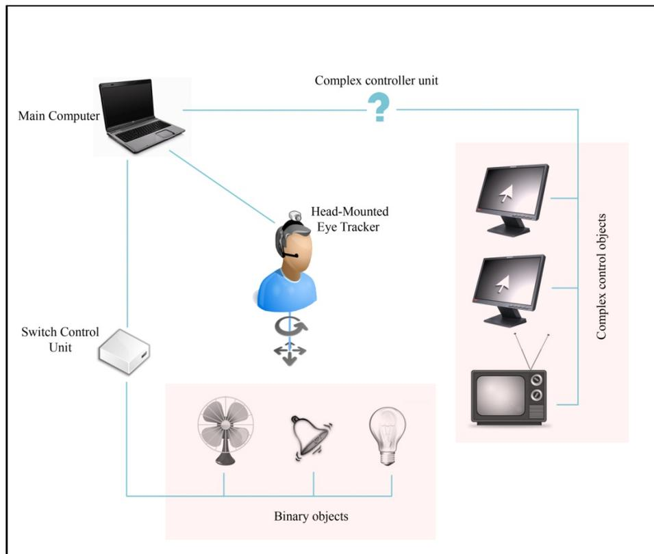
Figure 2: Schematic diagram of Gaze Environment control
